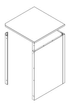
Attach the cover to the back panel structure with 8 truss head screws
