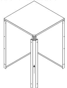
Screw the adjustable foot into the corner element – back element
