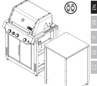
Install only one door module or case base on the corner module for this assembly variant!
